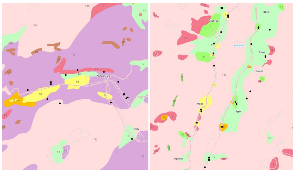
Figure 7.4: Example of landslide point data from “dataset 1” together with the quaternary deposit. “March 2014” event in Nordheimsund on the left and “Dagmar 2011” in Sjørfjorden on the right (the right picture shows only 27 of the landslide points due to the resolution of the map).
