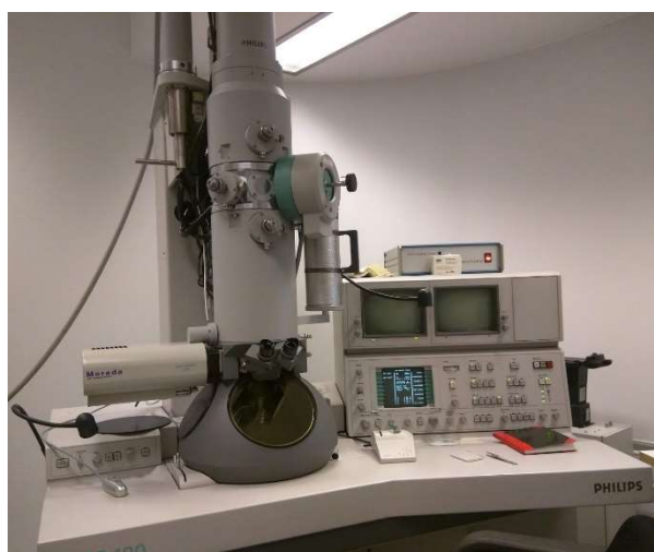
Figure 28: Photograph of the Philips FEI CM120 BioTwin transmission electron microscope located at the Institute of Oral Biology, University of Oslo.
