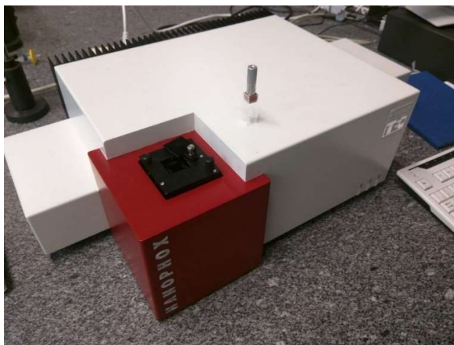
Figure 27: Photograph of the Nanophox DLS instrument at the Department of Chemistry, University of Oslo, and the type of cuvette used for measurements.
