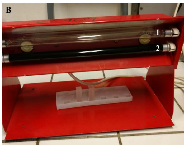
Figure 64. The UV lamps used for the thiyl radical-based charge tagging. Figure A shows a deuterium lamp. The sample was covered with the cardboard box observed in the back during irradiation. Figure B shows UV lamp 1 and 2 with unidentifiable wavelengths. Figure C shows the system set up during irradiation. The sample was covered with a cardboard box.
