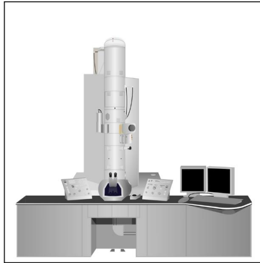
Figure 13: A representation of a JEOL 2100F depicting the TEM used during the experiments. The centerpiece is a large, vertical tube, containing the gun, lenses, detectors, and the sample.
