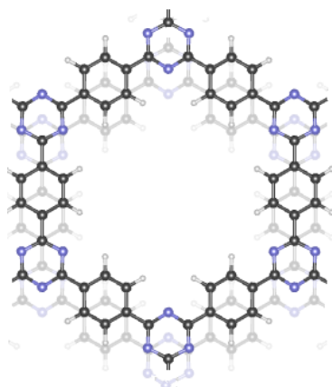
Figure 3.1: Illustrated here is one pore of optimally AA*-stacked CTF-1. Every layer is translated a fixed distance 1.82 Å compared to the next along one of the directions parallel to the linker as suggested by the stacking study results.
