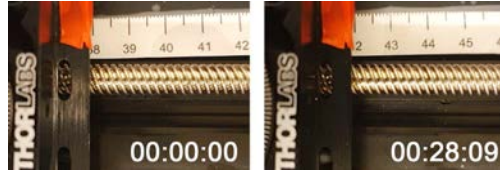
Figure 3.11: Screen shots from the clip shot by the mobile phone on the sled of the laser. The sled moved 4.00 cm in 28.09 seconds, putting the actual laser velocity at v_{laser} = 0.142 \text{ cm/s} .
