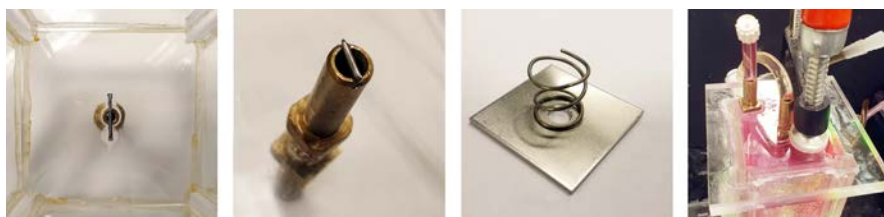
Figure 3.4: Some details from the cell design. In the first two pictures, we see pieces cut from needle tips, glued across the drain and inlet of the cell. At the inlet there is a nipple on both ends, to ensure that the flow commences inside the matrix. On the middle right there is a picture of the spring with a plate to jam the bead matrix in position. The plate has a hole that can be threaded over the injection nipple. To the right, we see an outlet valve to vent air from the cell.
