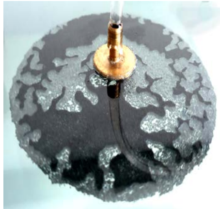
Figure 1.1: Picture from a quasi 2D experiment, conducted at Pore-Lab, with a Hele-Shaw cell, by Louison Thorens. The sample was prepared with a porous medium, saturated with dark liquid. The flow experiment was conducted by withdrawing liquid through a valve at the center of the sample. The air displaced liquid in fingers that formed a pattern, from the perimeter. Different flow rates produced different patterns.
