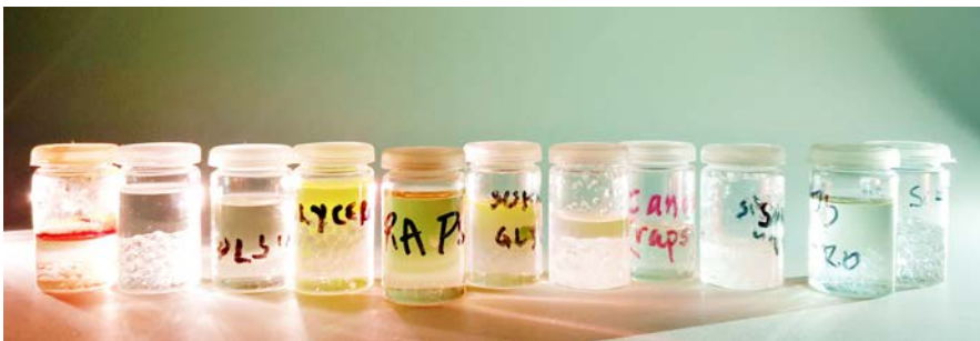
Figure 3.5: A selection of some of the liquids that were tested. Most were immediately discarded upon visual inspection, but the more promising candidates were put in the square-based container and scanned with the primitive set-up.
