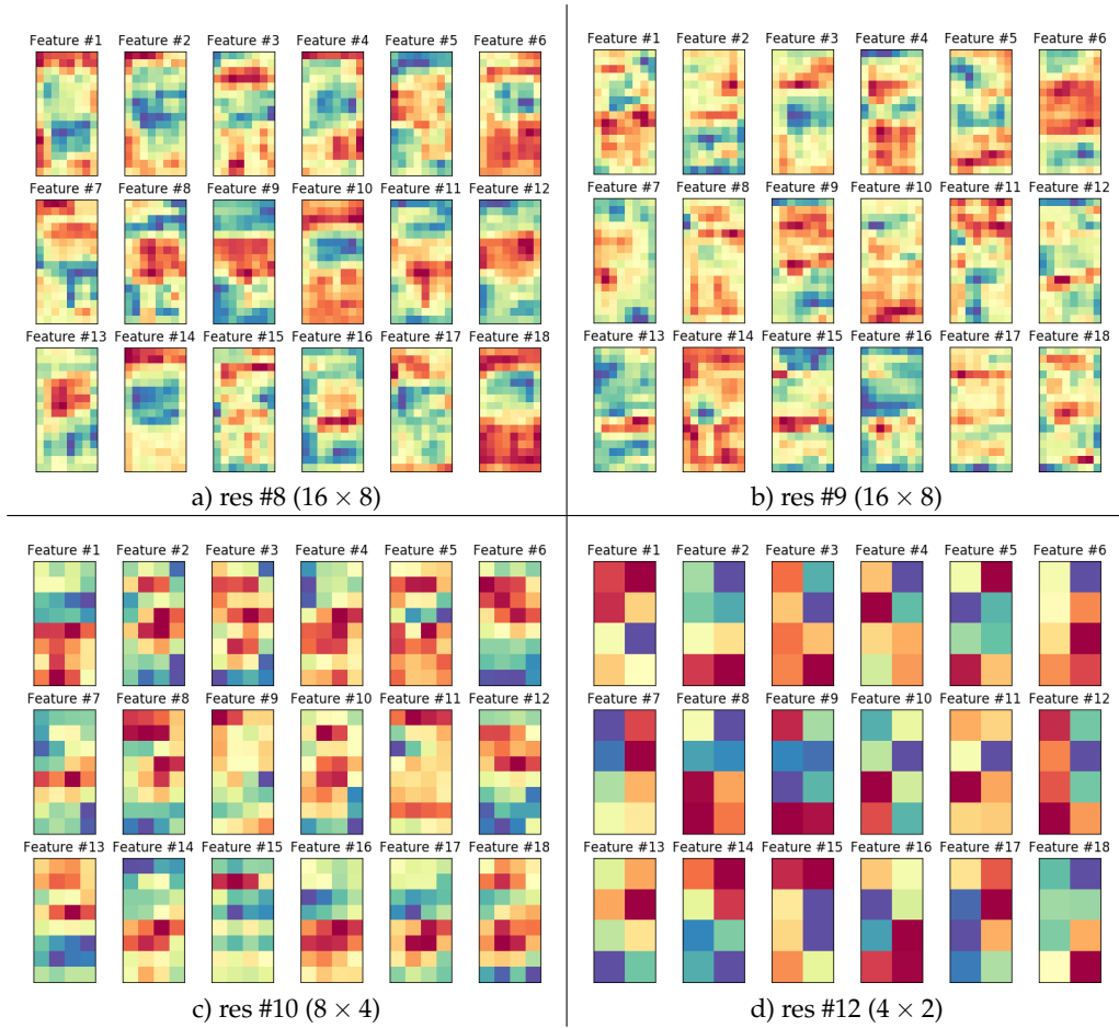
Figure 8.2: Continuation of Figure 8.1. 18 activation maps from a) the fourth residual block, b) the fifth residual block, c) the sixth residual block, and d) the seventh and final residual block. The dimensions of the respective activation maps are on the format H \times W .
