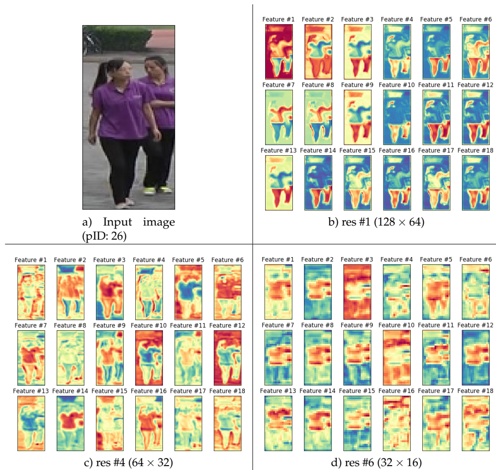
Figure 8.1: One input image (a) and 18 corresponding activation maps from b) the first residual block, c) the second residual block, and d) the third residual block. The dimensions of the respective activation maps are on the format H \times W . Continued in Figure 8.2.
