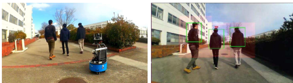
Figure 2.1: Left: a person-following robot. Right: the robot's field of view with the target to follow in the middle. Similar appearances due to clothing and hair color can make it challenging to distinguish between the target to follow and other people. Image from [53].
