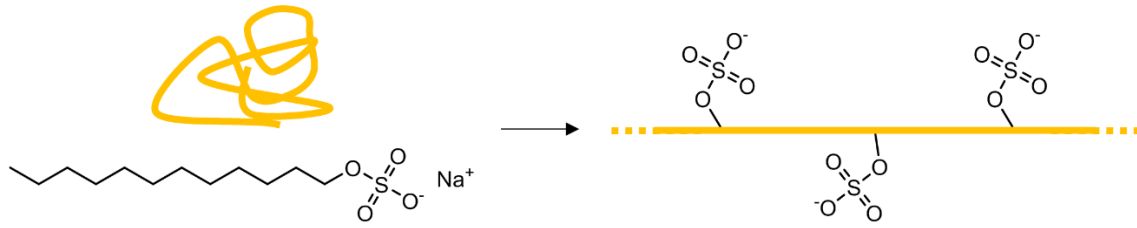
Figure 11: Denaturation of a protein by complexing with SDS forms a linear structure with a net uniformly distributed negative charge.
