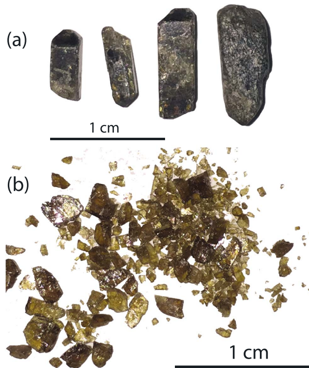
Figure 2. (a) Datas xenotime crystals are brown in color and have subhedral shapes. (b) XN02 crystal fragments (like those selected for the epoxy mounts and Isotope Dilution-Thermal Ionization Mass Spectrometry analyses) showing a brown-honey color.
