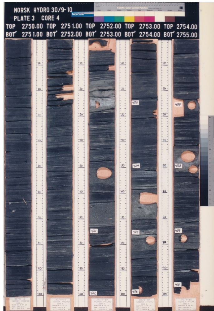
Figure 2.7: Core photograph of the Draupne Fm (2750-2755m MD) from well 30/9-10 (not included in this study. No core photographs of Hugin Formation from studied wells were available (Source: NPD, 2018).
