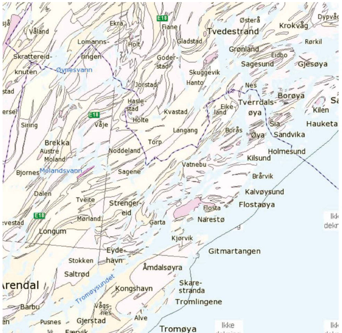
Figure 3.2.1: Part of a bedrock map covering the field area (scale 1:50,000). Crystalline rocks of the Bamble formation are found in this area. Most common are different types of granites (pink) and migmatites (yellow) (Padget 1988).
