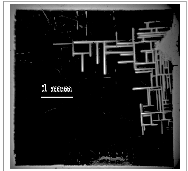
Figure 2: Magnetic flux pattern in superlattice B composed of 48 YBCO layers. The temperature of the sample at the record is 3.7 K. A magnetic field of 60 mT was applied after cooling sample in zero magnetic field.
