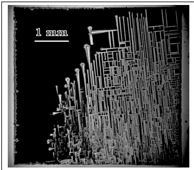
Figure 1: Magnetic flux pattern in superlattice A composed of 32 YBCO layers. The temperature of the sample is 3.7 K. A magnetic field of 60 mT was applied after cooling sample in zero magnetic field.
