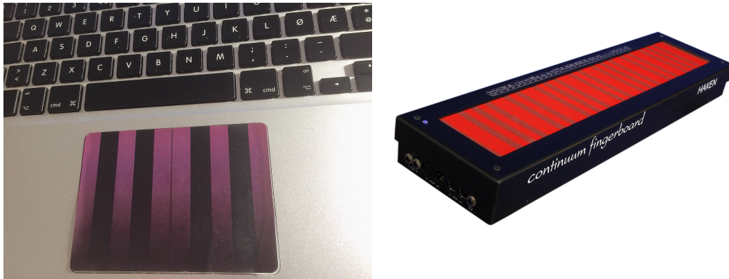
Figure 4.3.2.b To the left: A custom sticker on the trackpad surface visually mimics the playing surface of the Haken Continuum (right). The sticker reflects the pitch grid as depicted in Figure 3.2.2.
