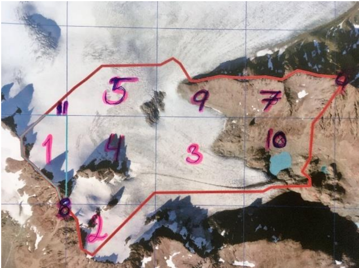
Figure 12: Grid cells used in the calculation in SeNorge, with the generated catchment area and an aerial photo of Koppangsbreen from 2016 as background layer
