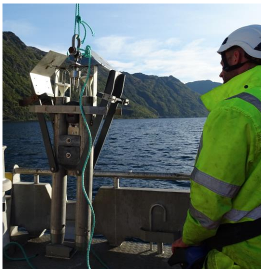
Figure 3.1.1: Gemini corer on deck in Øksfjord.
