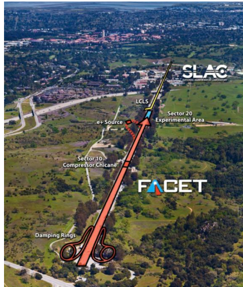
Figure 3.3: Bird's eye view and schematic layout of the FACET facility, using the first 2 km of the SLAC linac. Source: Mark Hogan, © SLAC.
