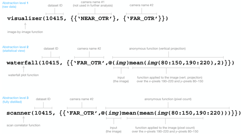
Figure B.3: Three-step code example based on the rapid-iteration data analysis tool. See Fig. B.2 for the corresponding output plots to lines 2 and 3. Note in particular the syntax similarity between the three functions—this helps to speed up the process of distilling the data, by allowing fine tuned inputs to be quickly moved to the next level of abstraction.
