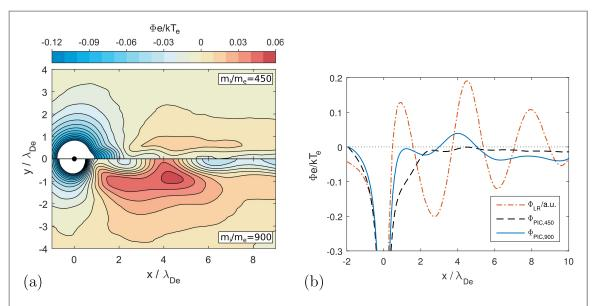
**Figure 2.** Potential distributions in x–y planes for  $\beta_i \approx 1.5$  and M = 1 for (a)  $m_i/m_e = 900$  and  $m_i/m_e = 450$ , as well as (b) along the x-axis through the center of the object. For comparison, the result from LR calculations (figure 6 in [33]) at the same  $\beta_i$  and M are also depicted in (b).
