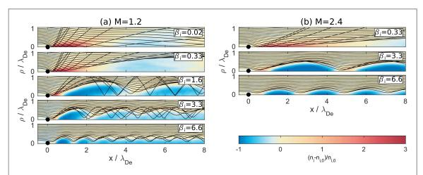
**Figure 3.** Test particle trajectories plotted on-top of normalized ion density distributions in the  $x-\rho$  plane (cylindrical symmetry) for M=1.2 (a) and M=2.4 (b) for different magnetizations  $\beta_i$ ;  $m_i/m_e=900$ . Only trajectories of ions entering the wake are shown.
