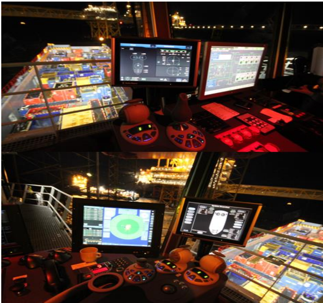
Figure 5: The DP system on both the left and right chairs. In the background are containers of different colours (the colours have no specific meaning). (Photo: Yushan Pan, 2015)
