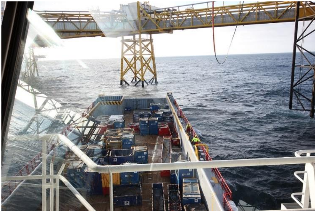
Figure 10: Shifting containers 5 and 6 under the deck while servicing the oil platform. Two deck crews check the pipeline and help to measure the distance between the vessel and the oil platform. (Photo: Yushan Pan, 2015)
