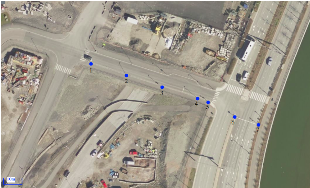
Figure 3.2: The blue dots mark the position and numbering of the passive samplers along Sørengkaia. Map from Statens Vegvesen's online service www.vegvesen.no/vegkart .
