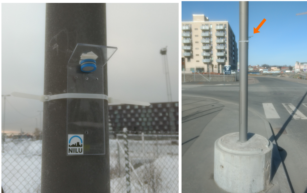
Figure 3.3: The pictures show a passive sampler on a plastic lid, attached to a lamp post.
