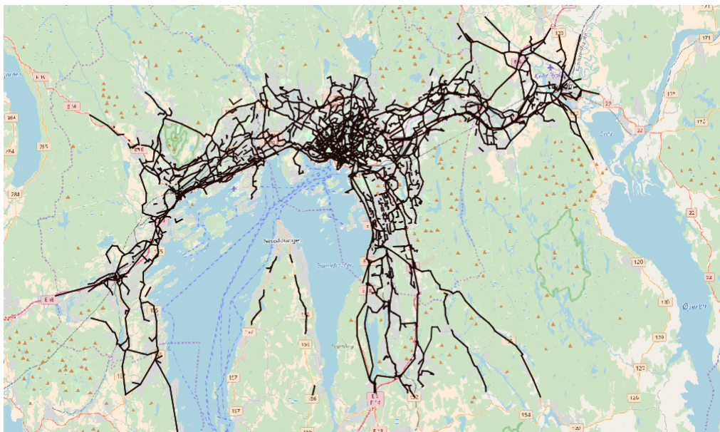
Figure 3.9: The lines represent the line sources used to model the emissions from roads with AADT > 1500 in the EPISODE runs.
