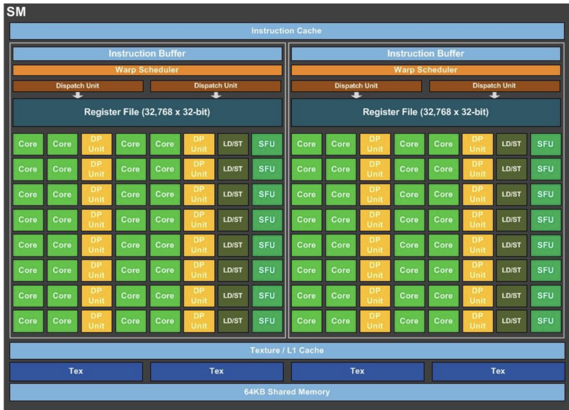
Figure 5: Pascal Streaming Multiprocessor
