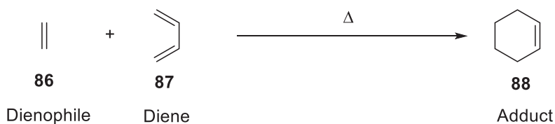
Scheme 10. The Diels-Alder reaction in its simplest form. Both the diene and the dienophile can be heavily substituted 16 .
