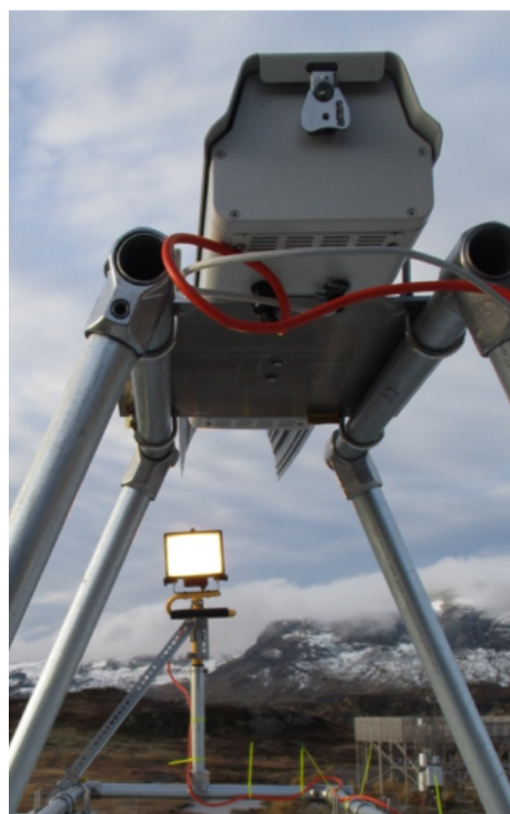
Figure 2.3.3: Precipitation Imaging Package at Haukelisetter mounted at the container pointing towards the double fence gauge.
