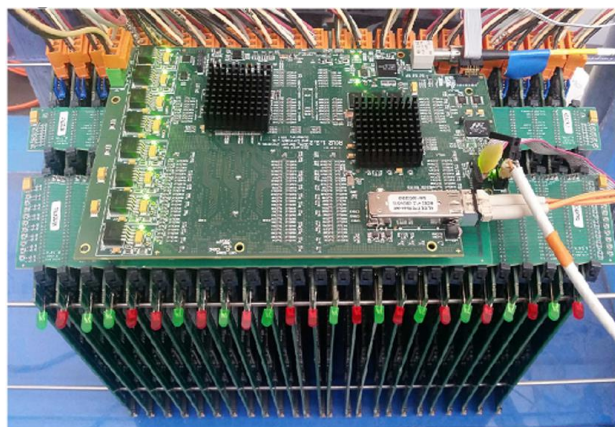
Figure 5-6 The CERN setup - 1 RCU2 connects to 25 FECs
