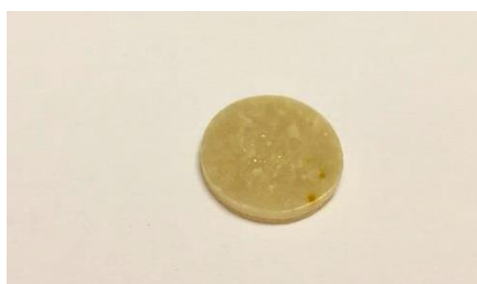
Figure 6.2: An image of ZnO ss0 was taken to illustrate the colour of ZnO pellet if not exposed to any additional treatment than pressing and sintering. The powder was white before sintering and obtained a pink colour after sintering. Some additional dark orange spots were observed close to the edge.
