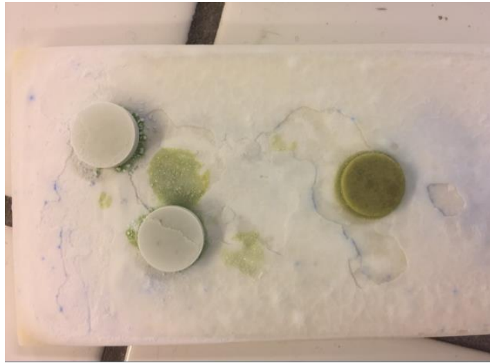
Figure 6.5: Image taken of the crucible and samples after sintering showing a white \text{ZnAl}_2\text{O}_4 layer on the samples with 5 mol% Al and the crucible, while the pure ZnO sample (to the right) doesn't have any additional powder.
