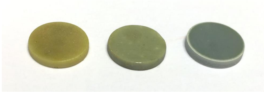
Figure 4.8: Samples prepared by solid-state synthesis with planetary ball milling shown the colour difference, ZnO_ssp (left): yellow/brown, 1ssp (middle): green and 5ssp (right): grey.
