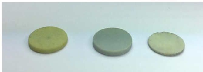
Figure 4.1: Samples prepared by sol-gel, ZnO_wc (left), 1wc (middle) and 5wc (right), are shown to illustrate the colour difference .
