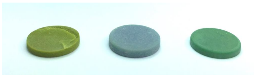
Figure 4.18: Samples prepared by solid state synthesis with roll ball milling, ZnO_ssr (left), 1ssr (middle) and 5ssr (right), are shown to illustrate the colour difference.
