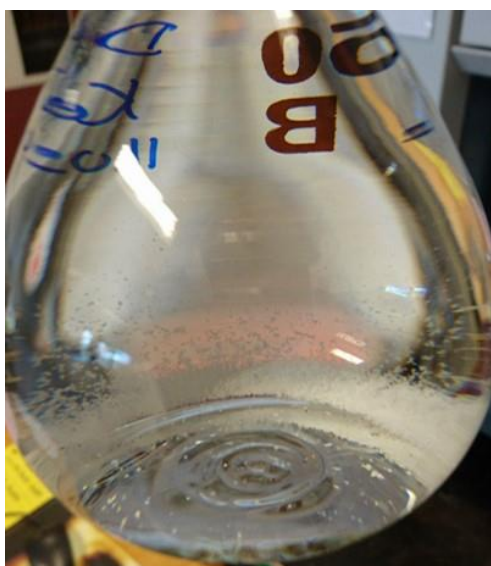
Figure 6 The ash sample after decomposition with HCl and HNO 3 (without HF) (Photo: J. Kessel)
