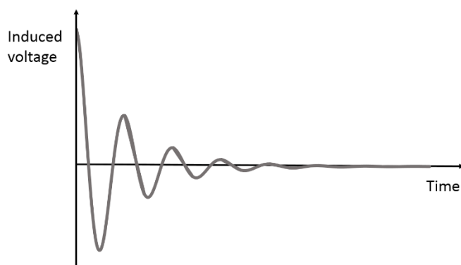
Figure 3.9: Schematic illustration of the free induction decay (FID) signal, which is recorded during an NMR experiment.
