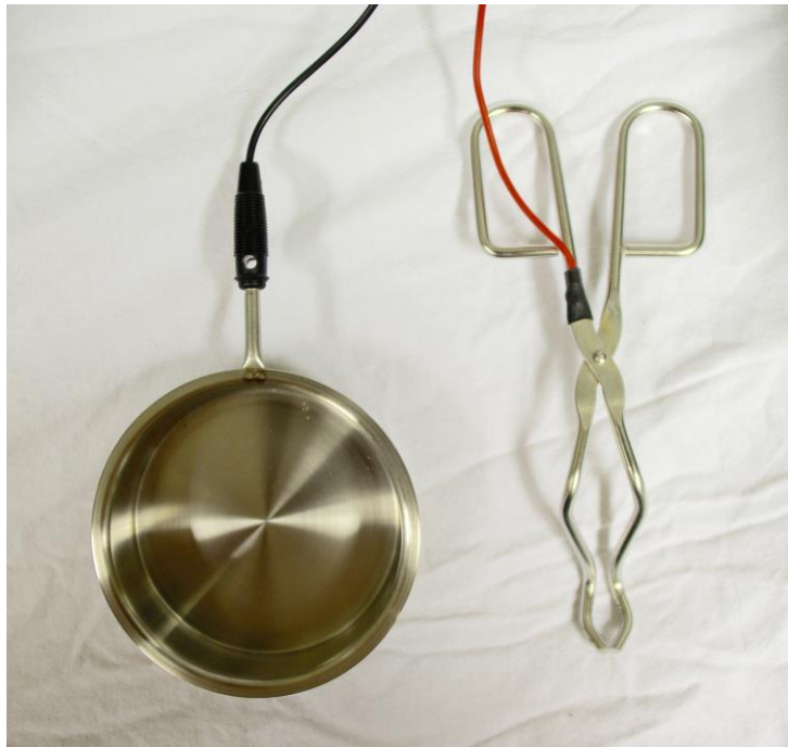
Figur 3.2: Image of the external etching equipment for the Lectropol-5.
