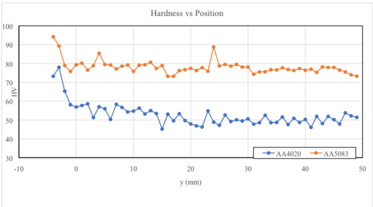
Figure 5.7: Compared hardness measurement graphs, as function of the position, of the AA4020 alloy (blue) and AA5083 alloy (orange). The position of the base plate (of alloy AA5754), first, base, layer and last, cap, layer noted in the graph window, to ease the interpretation. The dashed vertical line indicates the border between the base material and the deposited material.
