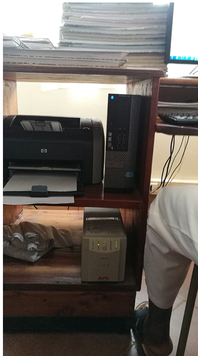
Figure 7.2: A desktop computer protected by an UPS.
