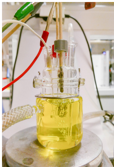
figure 24: Image of iron-copper solution during deposition.
