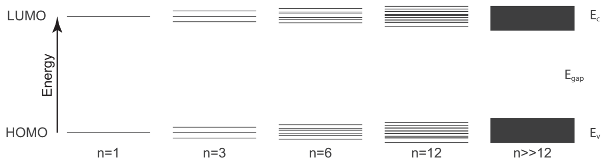
figure 2: Bonds to bands schematics of a typical system when similar atoms bond to form a bulk material where electron energies overlap to form bands of allowed energies.
