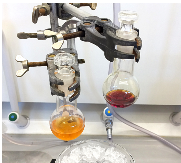
Figure 3.1: A successful chlorination of EDP (orange, left) and what is believed to be decomposed Cl-EDP (brown, right).
