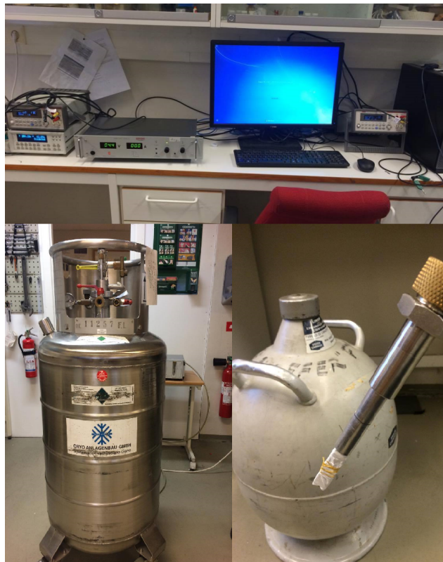
Figure 3.3: The figure shows the experimental setup for transport measurements at the superconductivity laboratory at the University of Oslo. The upper picture shows the power supply, the two multimeters and the computer used to process and control the measurements. The lower left picture shows the helium tank utilized, and the lower right picture shows the nitrogen dewar in the background and the sample mounted on the cryogenic rod in the front.
