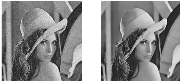
Figure 3.3: Image corrupted with white Gaussian noise with \sigma = 20 and PSNR = 17.9 (left) and its denoised version with PSNR = 32.7dB
