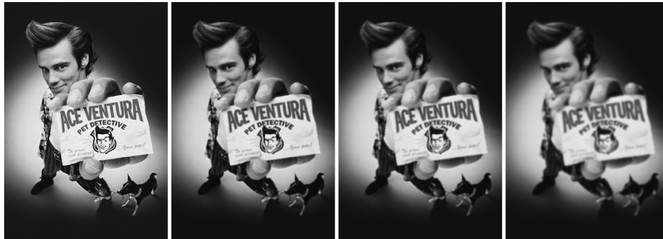
Figure 2.1: An example of Gaussian blurring an image. From left to right: the original image in grayscale, Gaussian filter with \sigma = 3 , with \sigma = 5 , with \sigma = 10 .
