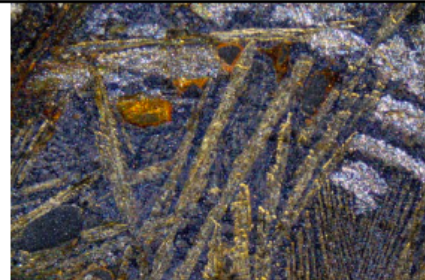
Fig. 26: As Fig 24, under OIL; crystalline laths are composed of 13.4% Si and 52.0% Fe (66.9% FeO).
