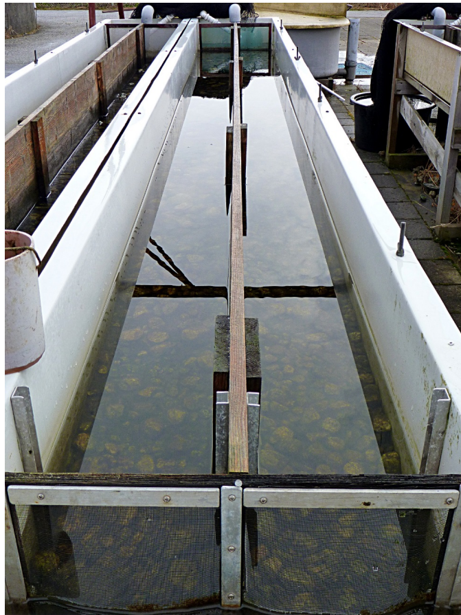
Figure 1. Photo of one pair of the artificial stream channels at normal water level during the summer trapping experiment. Top: water intake; bottom: Water outlet.
