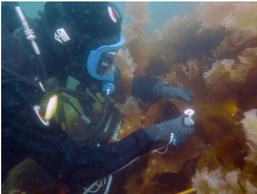
Figure 5: Photo illustrating how to measure the photosynthetic ability in situ with a Diving PAM-instrument. In this study, only ex situ measurements were taken. Photo: NIVA.
