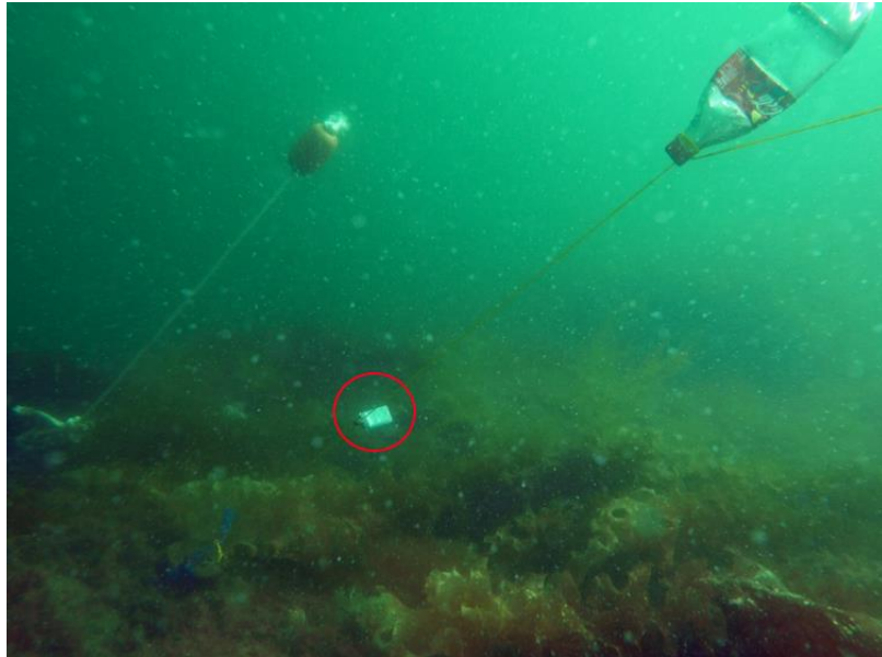
Figure 6: The setup of the HOBO-logger, measuring the temperature and light conditions. The logger can be seen as the small white square tied to the rope, close to the vegetation (red circle). The air-filled bottle maintained a vertical position and prevented the device from being overshadowed by the flora. Photo: NIVA.
