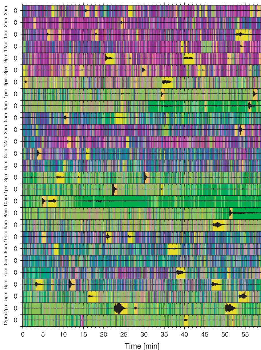
Figure 5. Vertical component seismograms of one array station for Merapi data for all analysed hours. Seismograms are bandpass-filtered between 0.3 and 19 Hz. Background colouring corresponds to cluster membership of each time window. SOM clustering and colours from Fig. 4(c) are used. Yellow time windows correspond to rockfall events and orange windows to volcano-tectonic events. Transition from greenish to bluish time windows reflects change in background wavefield due to human activity.
