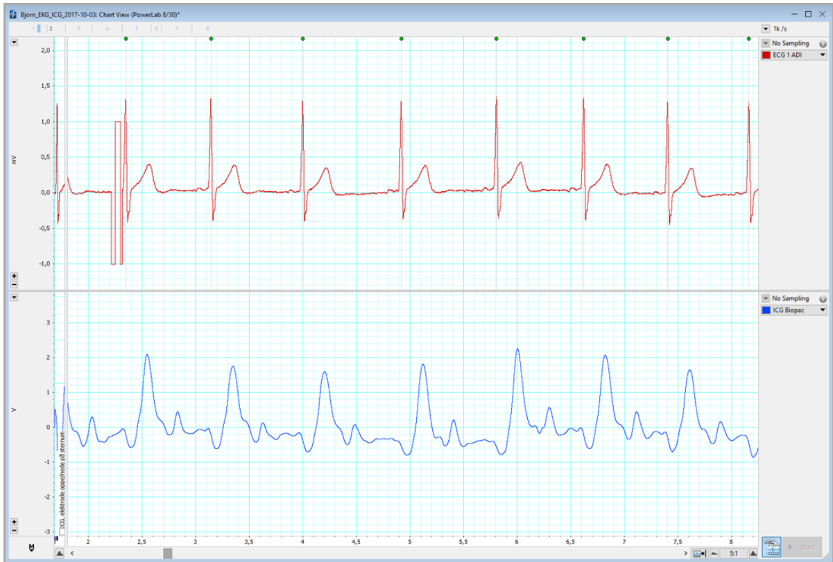
Fig.4.3.4: New electrode placement (fig.4.3.5), amplitude of ICG wave now greatly increased, making it much more distinguishable. Do note that the amplitudes of the peaks in-between the ICG did not drop, the picture is simply re-scaled.
