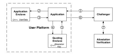
Figure 3.2: Attestation flowchart. The Challenger whats a Quote about the Application Enclave running on the User Platform. The Applications facilitates the attestation process. The Quoting Enclave signs the attestation report from the Application Enclave. The Challenger verifies the Quote before trusting the Application Enclave. [31]
