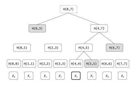
Figure 2.4: A Merkle Tree. The figure shows the authentication of a value  $y_4 \in Y = (y_0, \ldots, y_7)$ . The dotted node is the root tree hash and is a unique representation of all the leaf nodes ( $y_0$  to  $y_7$ ) in the tree. The drawn edges represent the sub-tree needed to authenticate  $y_4$ . The dark nodes are the values needed to create the sub-tree.
