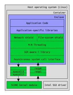
Figure 5.1: The SCONE architecture (green). The host OS uses a custom kernel module to execute system-calls on behalf of the SCONE container. The container runs the SGX enclave (blue) that contains the application. The enclave also contains the I/O shields, a thread scheduler, a minimal C library and a system-call dispatcher. [3]
