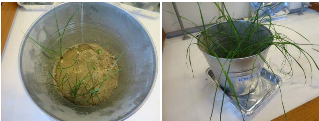
Figure 41 Ryegrass yield in two pots. Left: ryegrass in the unamended comparison pot with spiked soil and ryegrass, replicate number 3 (pot SSR3). Right: ryegrass in pot amended with 1% rice husk biochar, replicate number 4 (1RR4)
