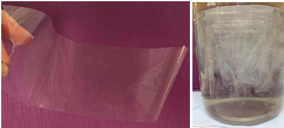
Figure 21 Polyethylene (PE) passive samplers used in the experiment. Left: a sheet of PE passive sampler. Right: 150 sheets of PE passive samplers stored in deionized water
