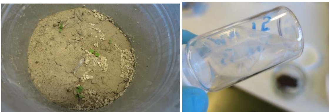
Figure 48 Left: PE passive sampler above the soil surface in the unamended comparison pot with spiked soil and PE passive sampler, replicate number 3 (pot SSPE3). Right: PE passive sampler from the pot with turnip, amended with 4% mixed wood biochar, replicate number 5 (pot 4MT5)
