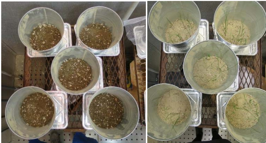
Figure 51 Pot with 0% biochar and ryegrass. Left: at start of trial. Right: three weeks into the trial, before irrigation
