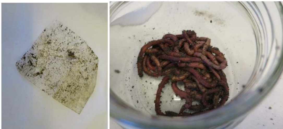
Figure 28 Left a sampled PE passive sampler before rinsing with deionized water. Right: Sampled earthworms prior to rinsing and depuration for 24 hours
