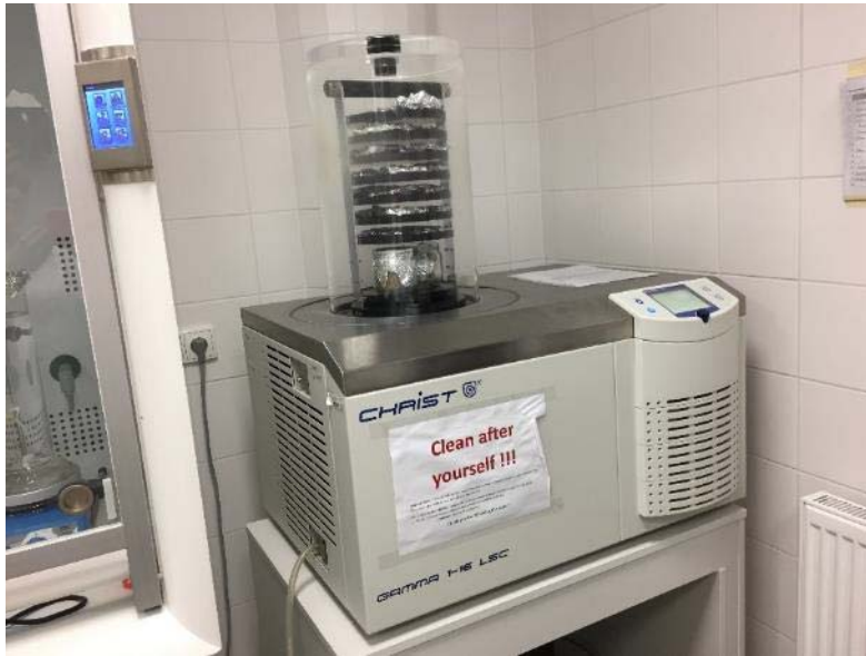
Figure 29 The Christ Gamma 1-16 LSC freeze dryer used to freeze dry the samples
