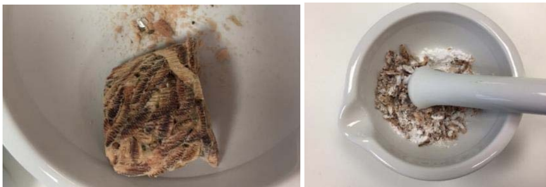
Figure 30 Left: freeze dried earthworms after weighing. Right: mixing of earthworms and sodium sulfate powder
