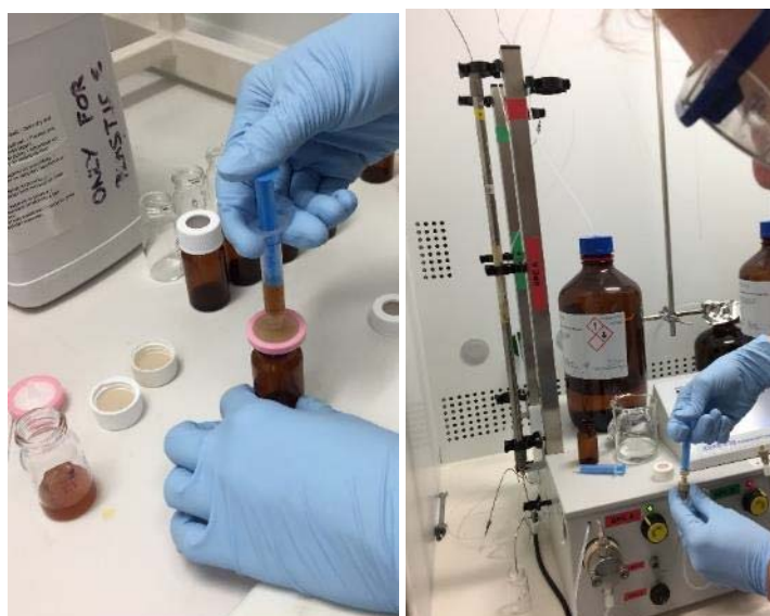
Figure 33 Left: filtering of an earthworm sample. Right: adding the filtered sample to the DeltaChrom KVAR 400 GPC-column
