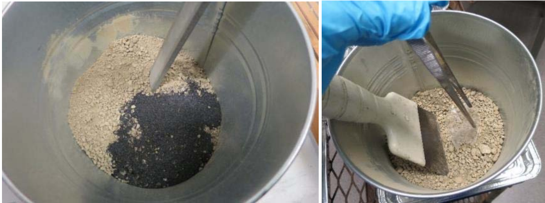
Figure 23 Left: biochar has been added to the pot, but not yet mixed in with the soil. Right: a PE passive sampler is placed on top of the soil before being pushed 4 cm below the soil surface
