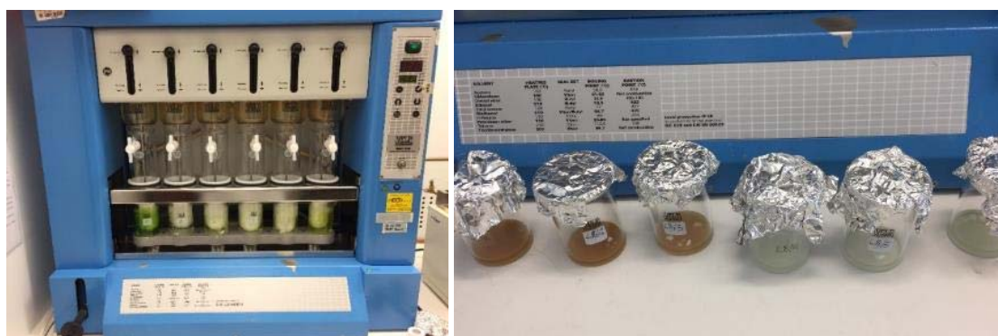
Figure 32 Left: VELP (SER 148/6) Randall Soxhlet instrument showing thimbles with plant samples immersed in solvent vials. Right: Samples of earthworms (brown colour) and soil after the extraction process
