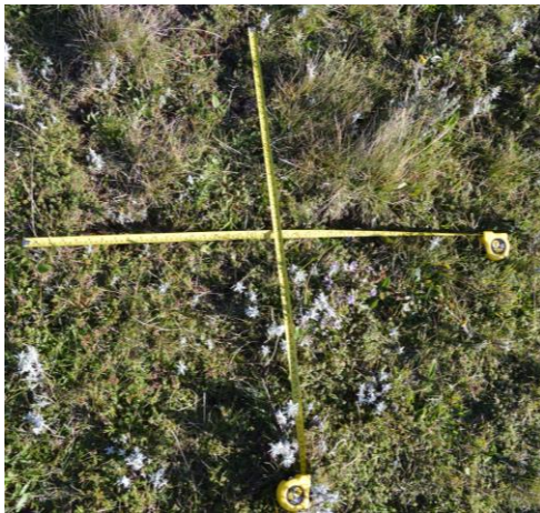
Figure 7. Method used to estimate ground cover in a patch.
