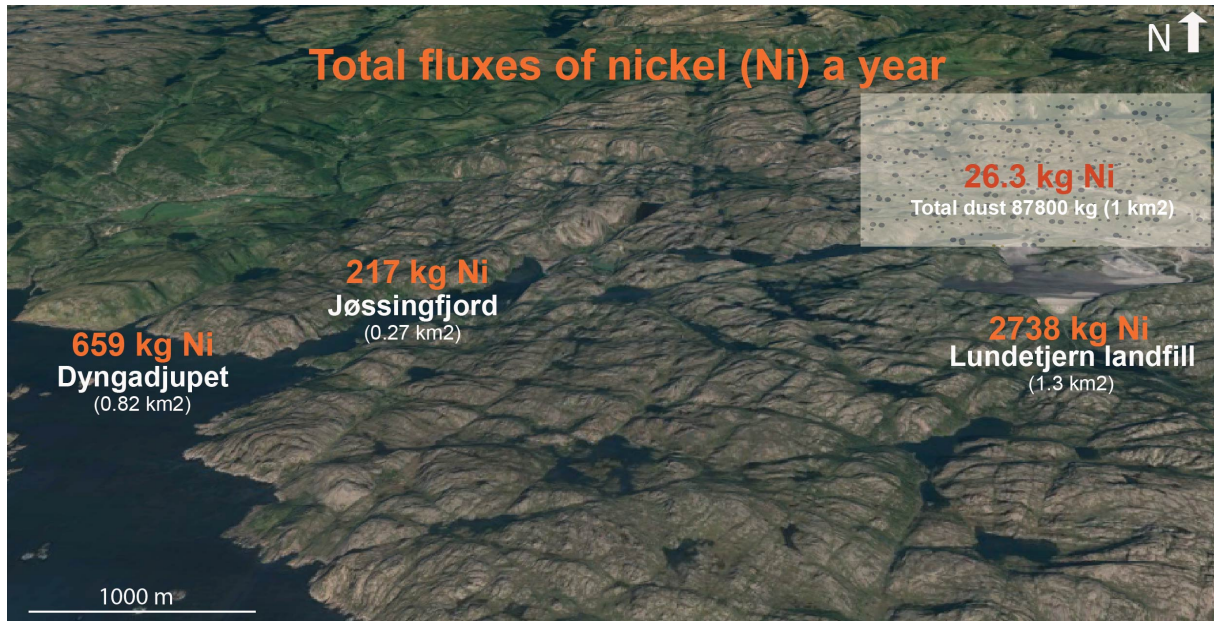
Figure 46 - Total fluxes of nickel (Ni) a year from Dyngadjupet, Jøssingfjord, Lundetjern landfill and from dust. The flux from Lundetjern is calculated from the concession limit of 7.5 kg/ day and not their actual leachate.
