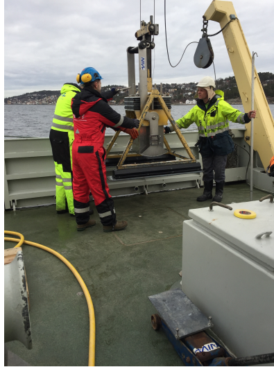
Figure 4.6: The box-corer reaching the boat deck with help from the boat crew and NIVA.
