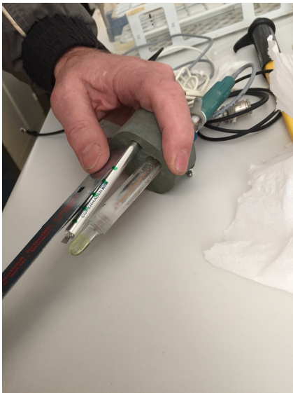
Figure 4.10: The reference electrode is marked with the depth intervals for analyses.
