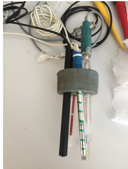
Figure 4.11: The electrode setup. The black electrode measured E_s , the red measured E_h and the see-through measured pH.
