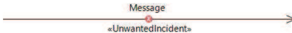
Figure 4.9: An example of a violated constraint with respect to the UnwantedIncident message.
