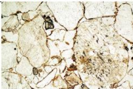
Fig. 25: Photomicrograph of M4040C (Subsoil); fine to coarse subsoil Bs horizon sands, with very thin organo-sesquioxidic grain coatings. PPL, frame width is ~2.38mm.
