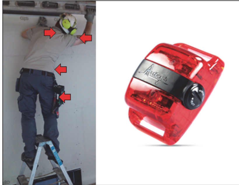
Photo. Left: Construction worker with Actigraph equipment during work (Photo, Lars-Kristian Lunde). Arrows mark Actigraph placements for units used in the papers presented in this thesis. Right: Actigraph GT3X+.
