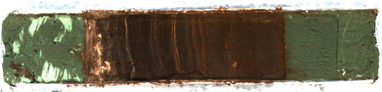
Figure 15) Picture of sediment core FLS113 (18.0 cm long), bottom side to the left, top to the right. The green on the top and bottom of the core is flower oasis.
