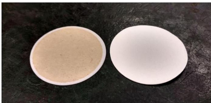
Figure 4.14: Picture of 0.2µm filters before (right) and after (left) filtration.
