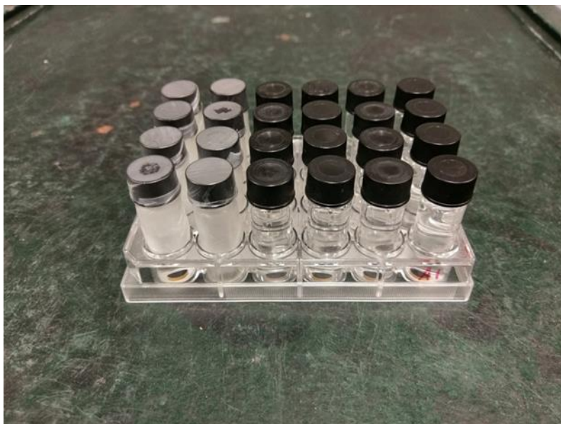
Figure 3.5: Illustration of how the vials were arranged on the SDR. All vials were sealed with parafilm before measurements.
