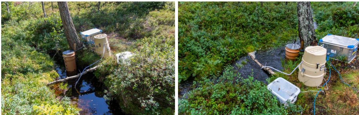
Figure 4.1 and 4.2: Photographs showing the water level before the episode (left) and at flow peak (right). Note the instrumental set-up with autosampler.
