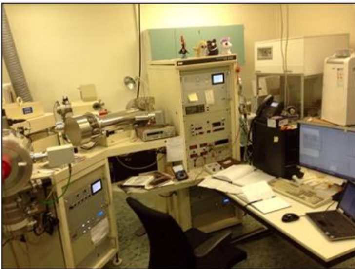
Figure 14 – TIMS machine. To the left is the source where the samples are introduced and the following pipes that the ionized elements will run through. To the right is the computer used to control all the processes in the machine.
