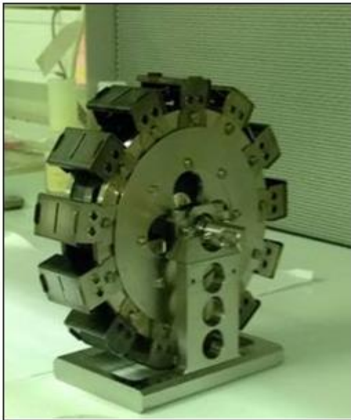
Figure 15 – turret for the samples to be placed on
