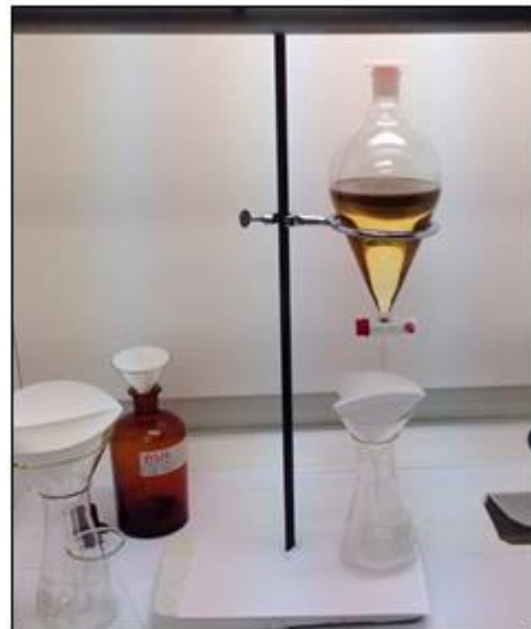
Figure 13 – picture of the heavy liquid bottle. Underneath is a bottle to collect the liquid the liquid that flows out. On top of this the paper that collects the heavy grain.. To the left is the bottle containing the heavy liquid.
