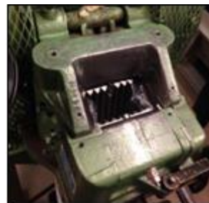
Figure 12 – “Jawcrusher”. In the middles is the bag that collects the sample. In front f the bag are the crushing plates that crush the rock
