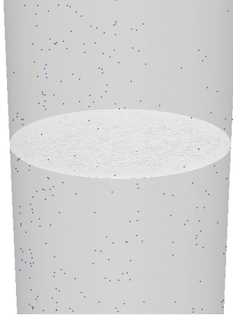
Figure 5.7: Particles moving very slowly in the viscous sublayer close to the boundary at T = 0.15s
